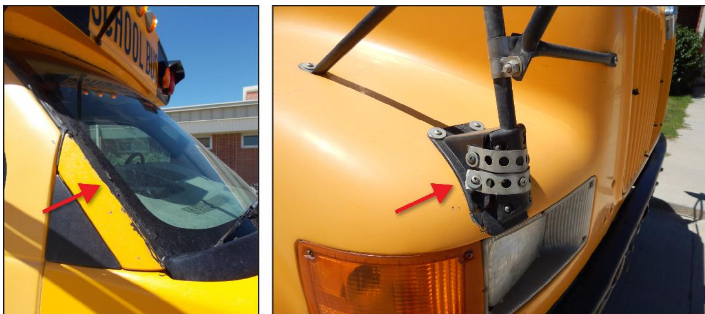
Figure 10: Windshield and Side Mirror Bracket Repairs on a School Bus Serving Routes on Gravel Roads on the Rosebud Reservation
